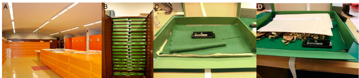
Figure 4 MEMORI measurement locations in the National Archives of Norway. (A) store room, (B) archive solid board boxes, (C) measurement in box without documents, and (D) measurement in box with documents.
