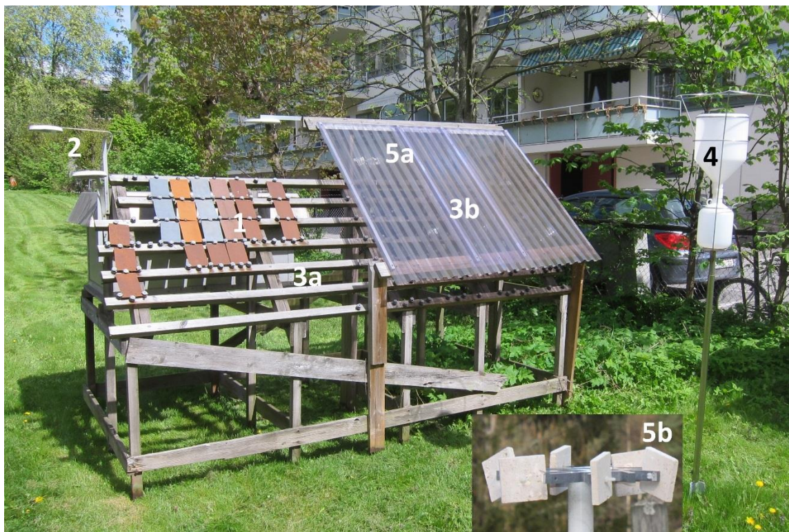
Figure 1: The ICP-materials station (no. 21, Appendix) located in the urban background in Oslo, Norway (2012). The picture shows metal plate samples in unsheltered position (1), holder disks for passive pollution samplers to the left on the rack (2), shelters for samples in a box behind the metal samples (3a) and under a plastic shield to the right (3b), and a precipitation collector to the very right on the photo (4). Limestone samples mounted on a carousel can be seen through the upper left corner of the plastic shield (5a) and in the low insertion (5b).
