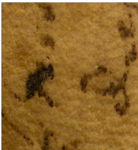
Figure 7b: Historical parchments (origin unknown): Movement of the fibre network may cause the stiff ink layer crack and flake off.
