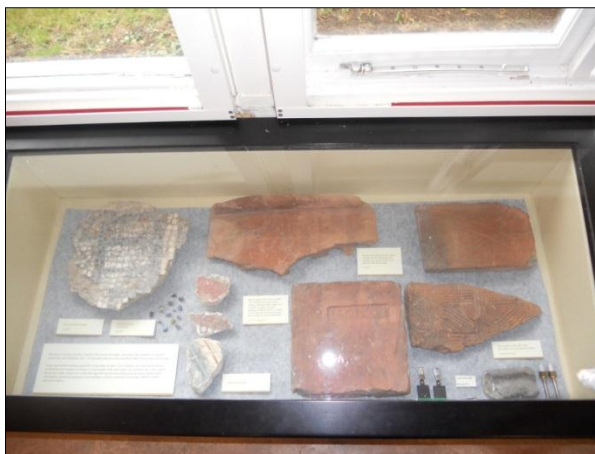
Figure 16: Showcase at Aldborough, with the charcoal cloth deployed. Air sampling devices are visible in the bottom right corner.
