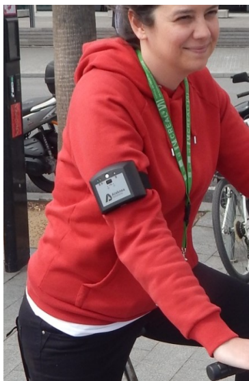
Figure 4.5: Example of a person carrying a LEO sensor platform on their arm.
