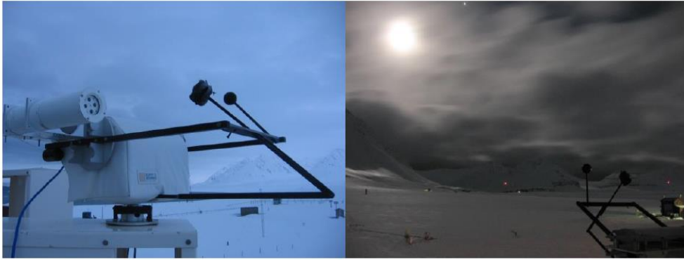
Figure 58: Moon PFR on the Kipp & Zonen tracker during the day (left, parking position) and during night-time measurements (right).
