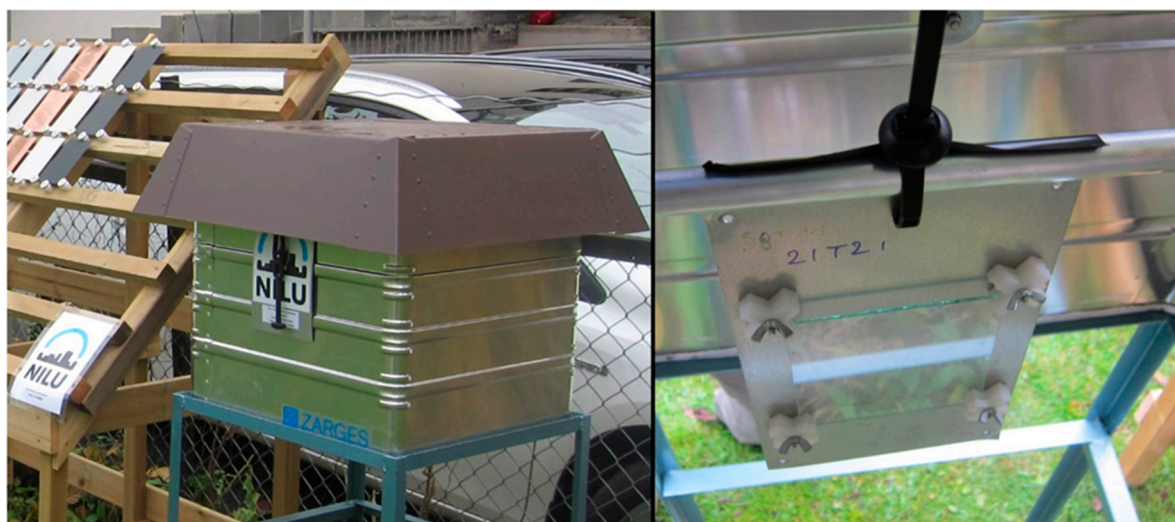
Figure 2. Soiling measurements on modern glass performed on the ICP-materials station in Oslo (2017) (The Oslo station is not included in Tables A1–A3, as particulate matter concentration was not measured at the station).
