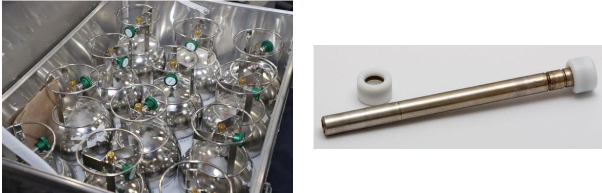
Figure 3: Samplers employed in the measurement campaigns. Canisters (left) and Tenax TA adsorption tube (right).
