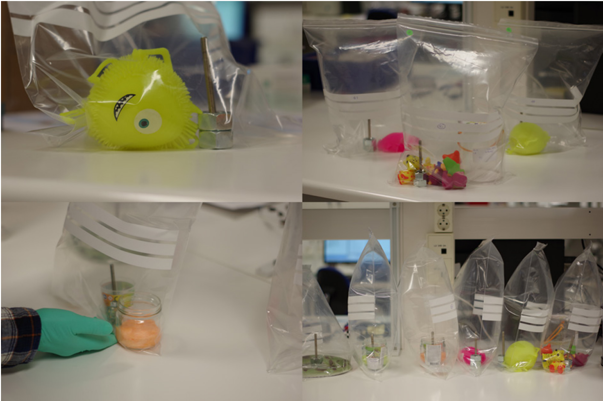
Figure 1 Part 1 – Measurements of VOC emissions in an inert atmosphere using Tenax TA passive air samplers.
