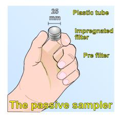
Figure 1: The passive sampler.
