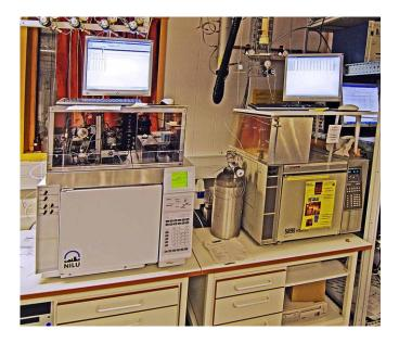
Figure 48: The new Gas Chromatograph for Methane and Nitrous Oxide measurements (left) side by side with the old system for Methane measurements.
