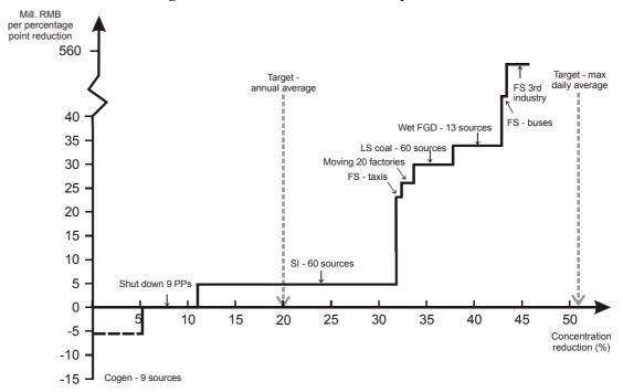
*Figure 1:Cost curve, SO<sub>2</sub> control options*
