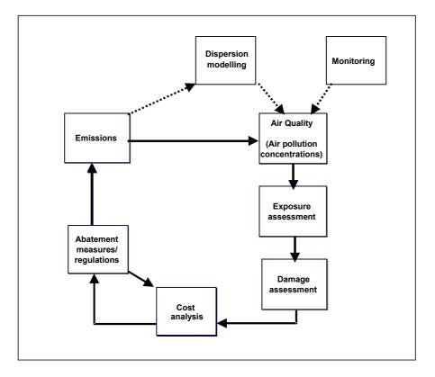
Figure 1: The system for developing an Air Quality Management Strategy (AQMS) based upon assessment of effects and costs
