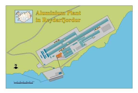
*Figure 7:* Layout of the aluminium smelter. 1) Potroom 1, 2) Potroom 2, 3), 4) and 5) Fume Treatment Plant (FTP 1, FTP 2, FTP 3), 6) Fume Treatment Carbon (FTC), 7) Green anode plant (GAP), 8) CastHouse
