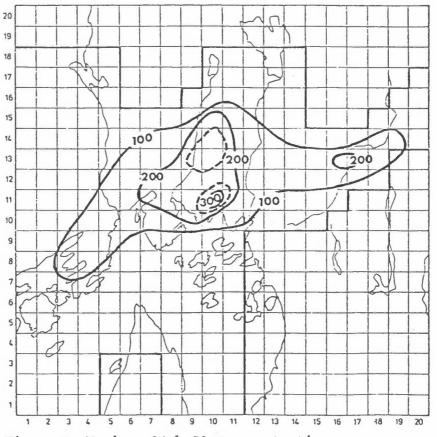
Figure 3: Maximum 24 h  $SO_{2^{12}}$  concentration. Unit:  $\mu g/m^3$ .
