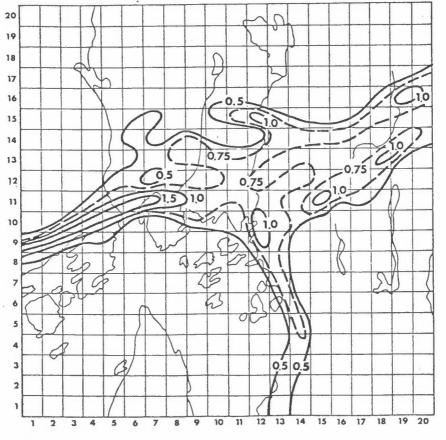
Figure 4: 3-month average for lead. Unit:  $\mu g/m^3$ . The calculations are based on a lead content in gasoline of 0.4 g per liter gasoline. For particulate matter/soot (24-h and 6-month averages), NO<sub>2</sub> (1-h and 6-month) and CO (1-h and 8-h values) it was found that one or several of the guidelines were exceeded by a factor of two in many street canyons. As an example, a map for 8-h average CO values is shown in Figure 5.
