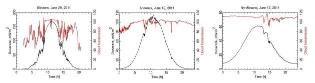
**Figure 20:** UV dose rates (left axis, black curves) and cloud transmission (right axis, red curves) during the days of maximum UVI in Oslo (left panel), Andøya (middle panel) and Ny-Ålesund (right panel). A cloud transmission of 100% represents clear sky conditions, whereas cloud transmissions of 20-30% represent heavy clouds.
