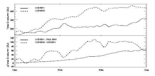
**Figure 13:** Modelled average column ozone north of 60°N for January, February and March 2010 (upper panel, dotted line) and 2011 (upper panel, full line) in simulations with no ozone-depleting chemistry north of 60°N. Relative difference in transport in 2010 compared to 2011 (lower panel, dotted line), and absolute ozone loss from heterogeneous chemistry in 2011 (lower panel, full line) (adapted from Isaksen, I., et al., to be submitted, 2012).
