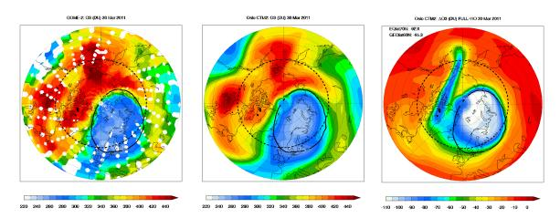
**Figure 12:** O3 column on 30 March 2011 as observed by the GOME-2 satellite instrument (left) and modelled by Oslo CTM2 (middle), and the corresponding column  $O_3$  loss (right) calculated as a difference between the full chemistry run and the run without chemistry north of 60°N. Black solid line is the 70°N equivalent latitude marking the vortex edge, while black dashed line is drawn at 60°N (Adapted from Isaksen, I., et al., to be submitted, 2012).
