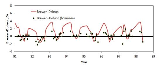
Figure 7: Monthly mean percentage difference between Brewer and Dobson 1991-1998. The red curve shows the original difference whereas the black dots represent the percentage difference after a seasonal correction factor is applied to the Dobson data.
