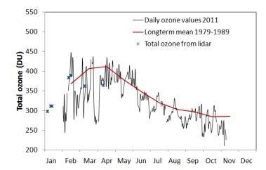
Figure 2a: Daily total ozone values measured at ALOMAR, Andøya, in 2011 by the Brewer/GUV instruments (black curve) and the LIDAR instrument (blue stars). The red line is the long-term monthly mean values from 1979-1989.
