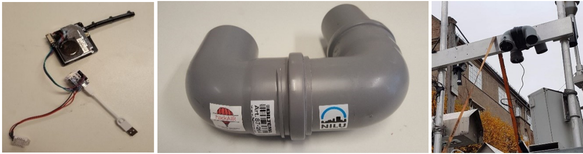
Figure 4: hackAIR stationary sensor system components (left), sensor casing (middle, modified from sensor.community sensor casing), and sensor co-located at one official air quality monitoring station in Oslo, Norway.
