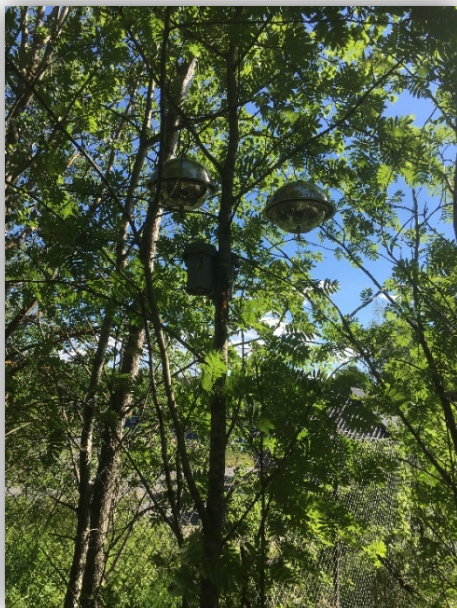
Figure 2. Air samples (PUF and XAD) installed at Grønmo site
