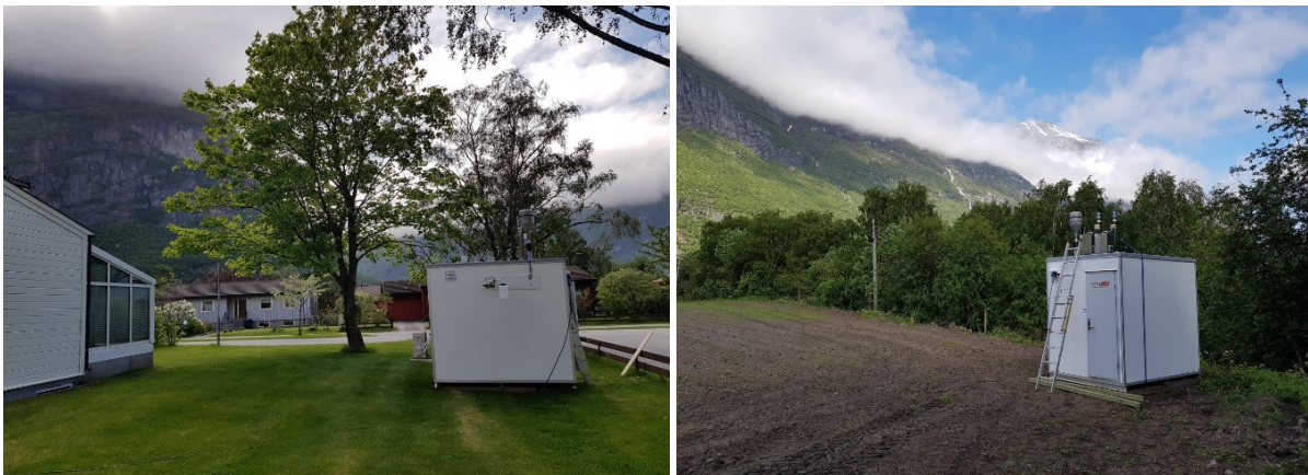
Figure 4: Sampling sites in the surroundings of the aluminium smelter Hydro Sunndal. Left: Pensjonistsenteret. The large intake above the roof is the intake for the PAH-sampler.
