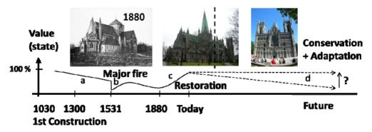
**Fig. 1.** The historical condition of the Nidaros cathedral in Trondheim, Norway, due to lacking maintenance (a), a catastrophic event (b), restoration (c) and future possible scenarios (d). The vertical dotted line distinguishes the front part (photo to the right) which was added during the conservation from the 1880s.
