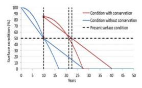
**Fig. 4.** Condition results diagrams for the Locomotive at Warsaw Railway museum, showing the assessment of past and future condition for the object structure and surface, based on the input from Table 1.
