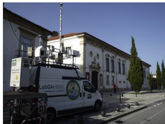
Fig. 2. Set-up of the AQ mobile station and micro-sensors during the 1st EuNetAir campaign.
