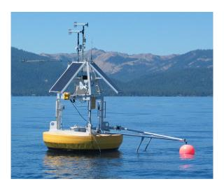
**Figure 4** – One of the four Lake Tahoe buoys measuring LST as well as a variety of meteorological parameters.
