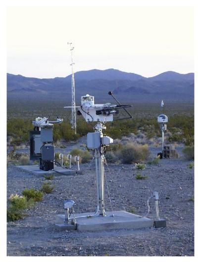
**Figure 6** – Example of a SURFRAD station, here showing the Desert Rock (Nevada) station. Clockwise from left center: Radiometer platform, met tower, total sky imager, and solar tracker. From http://www.esrl.noaa.gov/gmd/grad/surfrad/.
