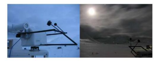
Figure 49: Moon PFR on the Kipp & Zonen tracker during the day (left, parking position) and during night-time measurements (right).
