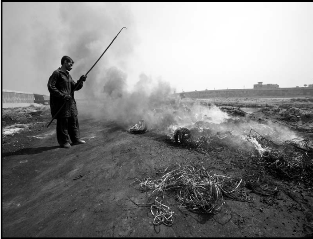
Figure S1 (a): Open burning of wires to retrieve metal in Shershah, Karachi ( Liyari river can be seen at the back which is ultimate dumping site for all types of waste) (Photo: Giovanni Porzio)
