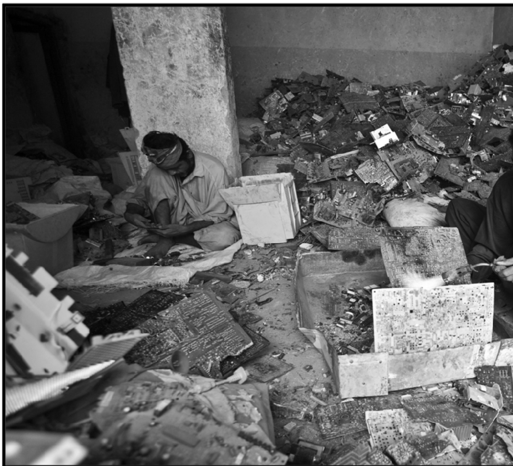
Figure S1 (c): Extraction of valuable materials through blow torches and physical disintegration, Karachi (Photo: Giovanni Porzio)
