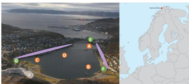
**Figure 1:** The sampling sites in Storvannet (A-D), inflowing (F and G) and outflowing (E) rivers. Direct emissions of sewage occurred earlier at site D. The shaded areas indicate where sewage leaks and overflows are known to occur. The right-hand map shows the location of Hammerfest.
