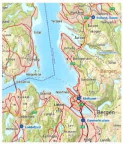
Figure 1: Air monitoring stations in Bergen
