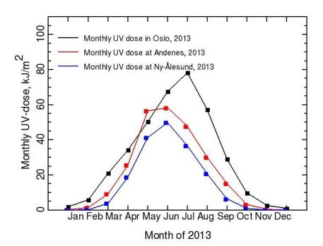
*Figure 17:* Monthly integrated UV doses (in  $kJ/m^2$ ) in 2013 measured with the GUV instruments located in Oslo, at Andøya and in Ny-Ålesund.
