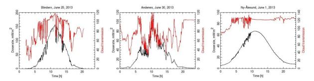
*Figure 16:* UV dose rates (left axis, black curves) and cloud transmission (right axis, red curves) during the days of maximum UVI in Oslo (left panel), Andøya (middle panel) and Ny-Ålesund (right panel). A cloud transmission of 100% represents clear sky conditions, whereas cloud transmissions of 20-30% represent heavy clouds.
