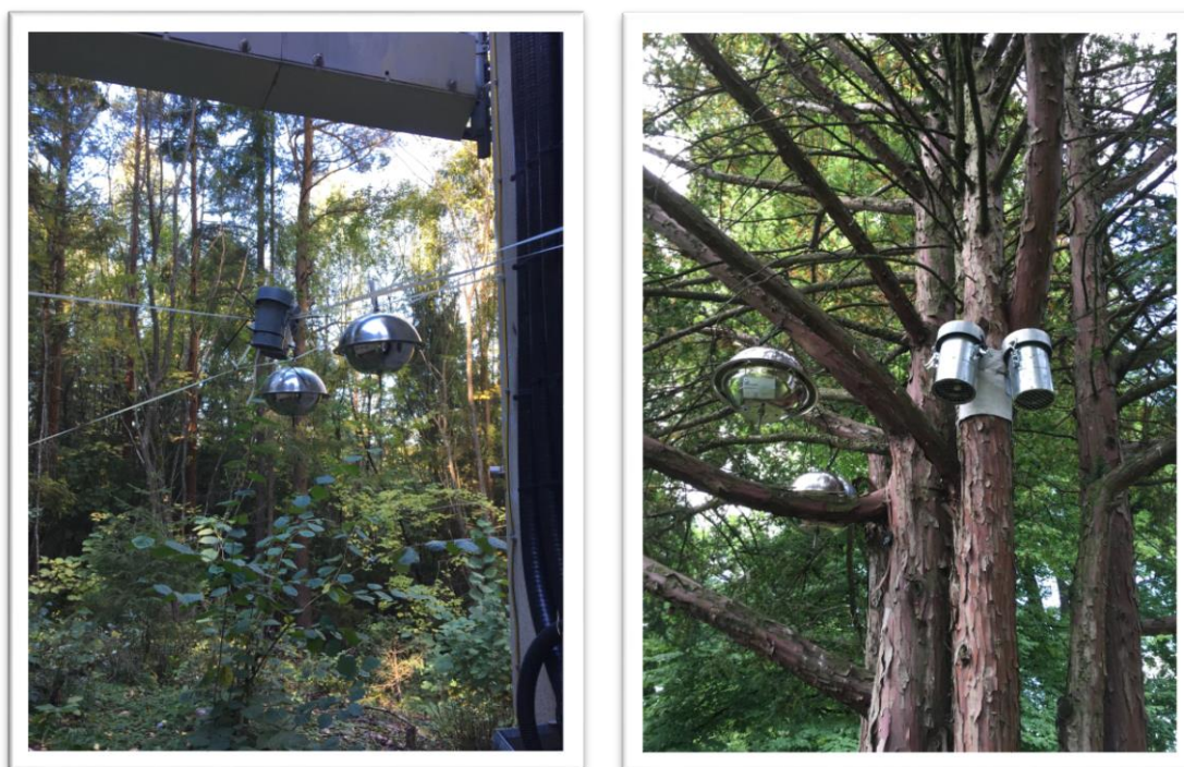
Figure 1. Air samples (PUF and XAD) at two sampling sites, VEAS site to the left and Slottsparken to the right.
