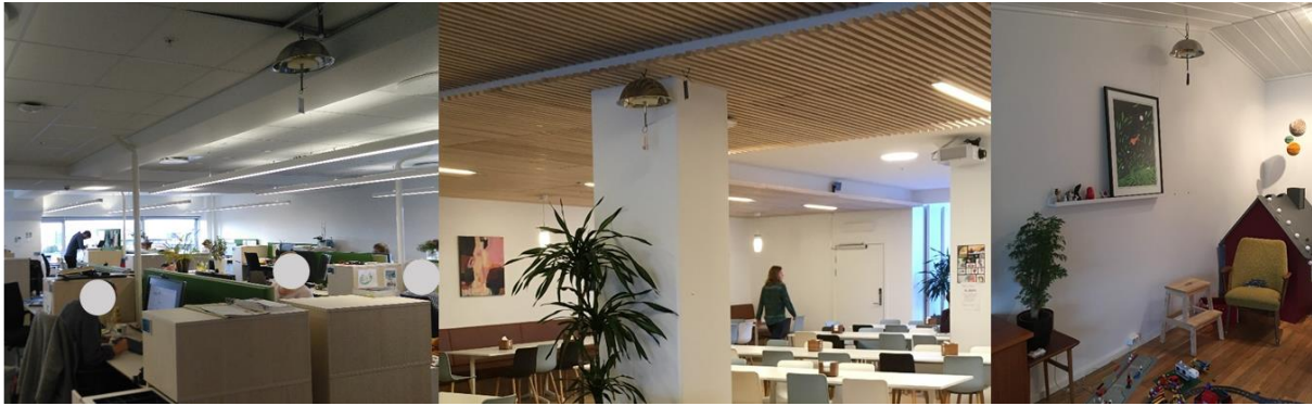
Figure 1: Air sampling equipment: PUF-PAS (top) and XAD-PAS (bottom), used to perform screening in indoor residential and non-residential environments.
