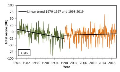
Figure 4b: Variation in total ozone over Oslo/Kjeller for the period 1979–2019 after the seasonal variations have been removed. The green line represents measurements performed with the Dobson instrument, whereas the orange line represents Brewer measurements. Trend lines are marked as black lines.
