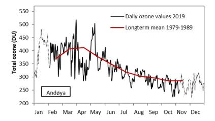
Figure 2a: Daily total ozone values measured at ALOMAR, Andøya, in 2019 by the Brewer and GUV instruments (black curve). The red line is the long-term monthly mean values from 1979-1989. The dotted line represents GOME2 satellite measurements.
