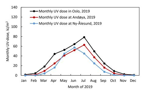
Figure 18: Monthly integrated UV doses (in  $kJ/m^2$ ) in 2019 measured with the GUV instruments located in Oslo, at Andøya and in Ny-Ålesund.
