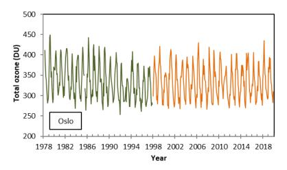
Figure 4a: Time series of monthly mean total ozone in Oslo and at Kjeller 1979-2019. The green line represents measurements performed with the Dobson instrument, whereas the orange line represents Brewer measurements.
