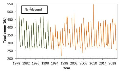
Figure 6a: Time series of monthly mean total ozone at Ny-Ålesund 1979–2019. The green line represents total ozone data from satellite, whereas the orange line represents measurements from ground-based instruments.
