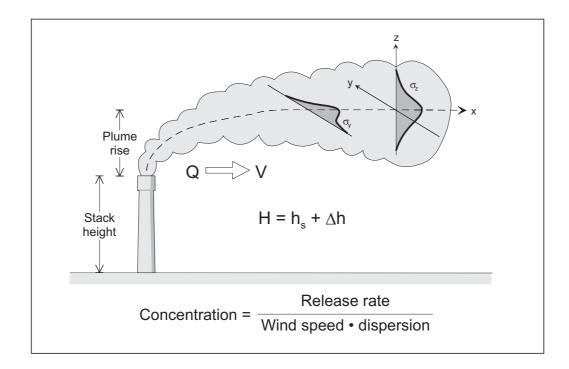
Figure 24: Gaussian point source geometry.
