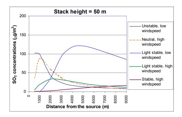
Figure 7: Maximum one-hour concentration of  $SO_2$  in  $\mu g/m^3$  at ground level, as a function of distance to the source, for different meteorological conditions, for a stack height of 50 m, Phase 2.
