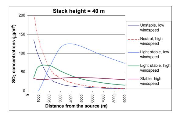
Figure 4: Maximum one-hour concentration of  $SO_2$  in  $\mu g/m^3$  at ground level, as a function of distance to the source, for different meteorological conditions, for a stack height of 40 m, Phase 1.
