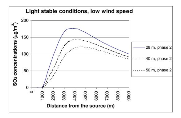
Figure 12: Maximum one-hour concentration of  $SO_2$  in  $\mu g/m^3$  at ground level, as a function of distance to the source, for different stack heights for Phase 2, under light stable conditions and low wind speeds.
