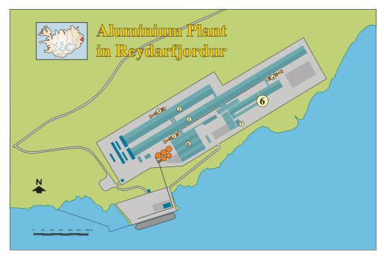
*Figure 1:* Layout of the aluminium smelter. 1) Potroom 1, 2) Potroom 2, 3), 4) and 5) Fume Treatment Plant (FTP 1, FTP 2, FTP 3), 6) Fume Treatment Carbon (FTC), 7) Green anode plant (GAP), 8) CastHo
