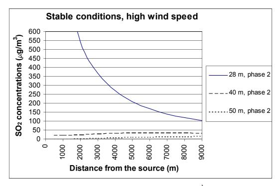
Figure C: Maximum one-hour concentration of  $SO_2$  in  $\mu g/m^3$  at ground level, as a function of distance to the source, for different stack heights for Phase 2 and under stable conditions and high wind speeds. For a 28 m stack the calculated maximum one-hour concentration of  $SO_2$  is 950 and 1450  $\mu g/m^3$ , at 1000 m and 500 m from the source, respectively.
