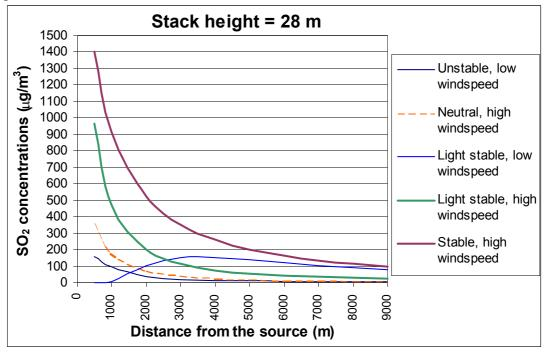
Figure 2: Maximum one-hour concentration of  $SO_2$  in  $\mu g/m^3$  at ground level, as a function of distance to the source, for different meteorological conditions, for a stack height of 28 m, Phase 1.
