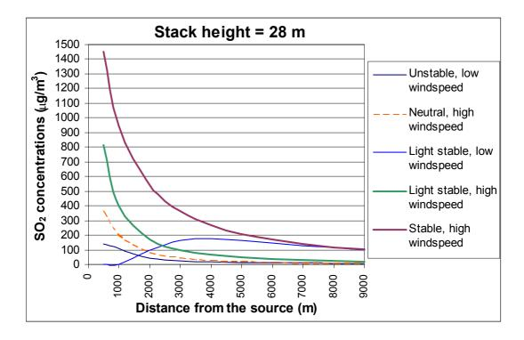
Figure 3: Maximum one-hour concentration of  $SO_2$  in  $\mu g/m^3$  at ground level, as a function of distance to the source, for different meteorological conditions, for a stack height of 28 m, Phase 2.
