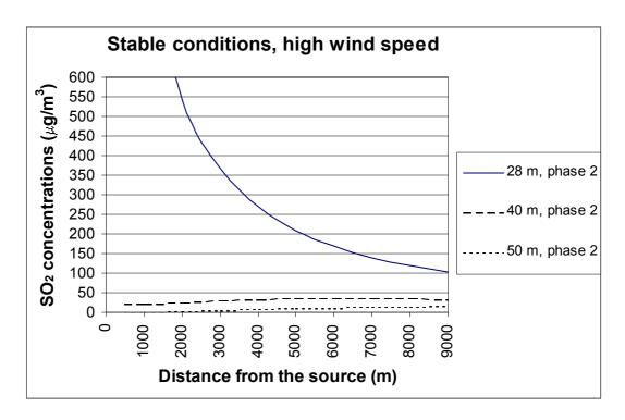
Figure 10: Maximum one-hour concentration of  $SO_2$  in  $\mu g/m^3$  at ground level, as a function of distance to the source, for different stack heights for Phase 2 and under stable conditions and high wind speeds. For a 28 m stack the calculated maximum one-hour concentration of  $SO_2$  is 950 and 1450  $\mu g/m^3$ , at 1000 m and 500 m from the source, respectively.
