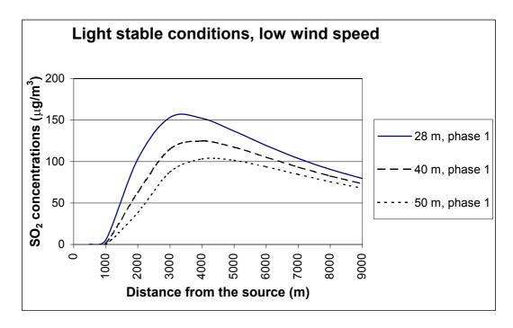
Figure 11: Maximum one-hour concentration of  $SO_2$  in  $\mu g/m^3$  at ground level, as a function of distance to the source, for different stack heights for Phase 1, under light stable conditions and low wind speeds.
