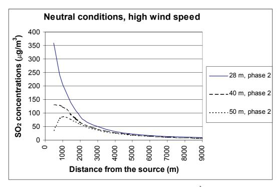
Figure A: Maximum one-hour concentration of  $SO_2$  in  $\mu g/m^3$  at ground level, as a function of distance to the source, for different stack heights for Phase 2 and under neutral stability conditions and high wind speeds.
