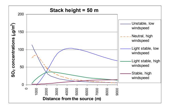
Figure 6: Maximum one-hour concentration of  $SO_2$  in  $\mu g/m^3$  at ground level, as a function of distance to the source, for different meteorological conditions, for a stack height of 50 m, Phase 1.
