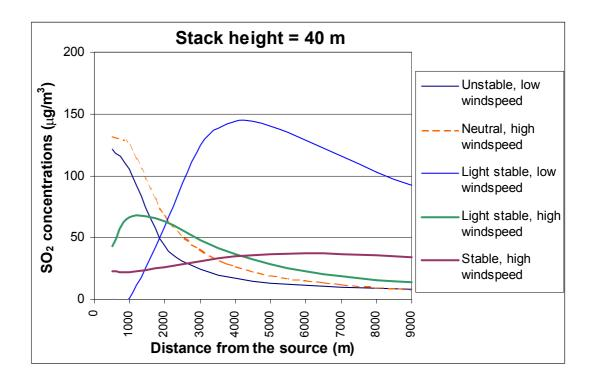
Figure 5: Maximum one-hour concentration of  $SO_2$  in  $\mu g/m^3$  at ground level, as a function of distance to the source, for different meteorological conditions, for a stack height of 40 m, Phase 2.
