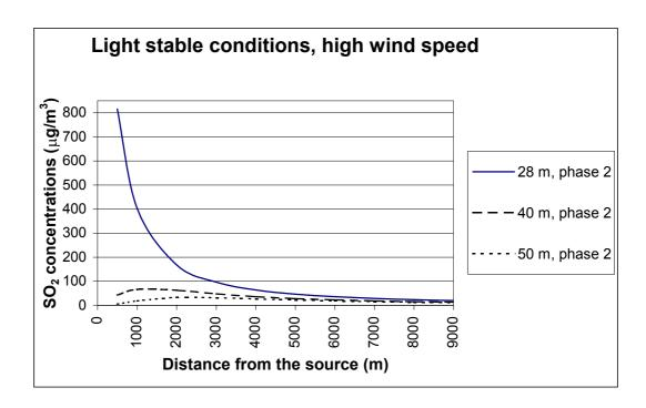
Figure B: Maximum one-hour concentration of  $SO_2$  in  $\mu g/m^3$  at ground level, as a function of distance to the source, for different stack heights for Phase 2 and under light stable conditions and high wind speeds.
