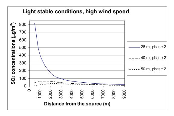
Figure 9: Maximum one-hour concentration of  $SO_2$  in  $\mu g/m^3$  at ground level, as a function of distance to the source, for different stack heights for Phase 2 and under light-stable conditions and high wind speeds.
