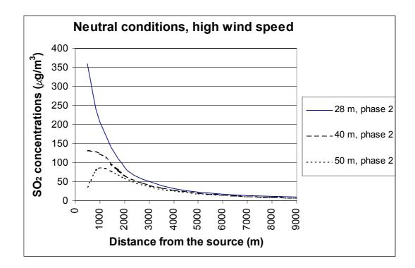
Figure 8: Maximum one-hour concentration of  $SO_2$  in  $\mu g/m^3$  at ground level, as a function of distance to the source, for different stack heights for Phase 2 and under neutral stability conditions and high wind speeds.
