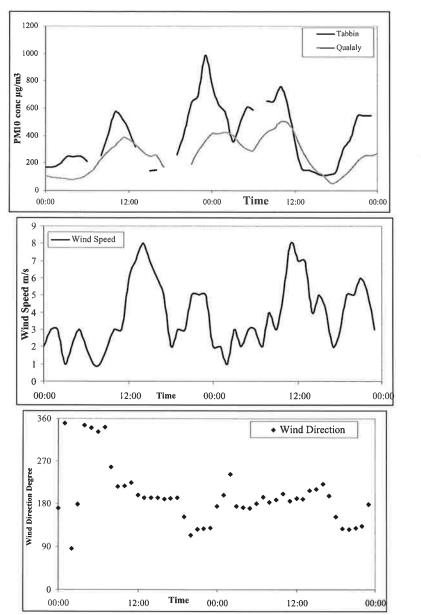
Figure 10:  $PM_{10}$  and wind measured at 11-12 April 2000.
