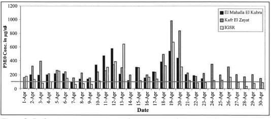
Figure 5: Daily average concentrations of PM<sub>10</sub> measured at IGSR - Alex, ElMehalla ElKubra and Kafr Elzayat stations (which represents Alexandria and Delta) in April 2000
