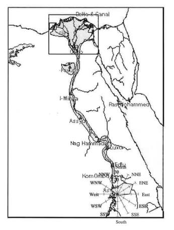
Figure 9: Wind frequency distribution in Upper Egypt during April 2000.
