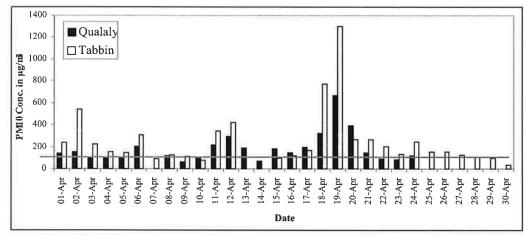
Figure 4: Daily average concentrations of  $PM_{10}$  measured at Tabbin and Kolaly stations (which represents Greater Cairo) in April 2000
