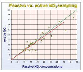
The integrated passive sampling of  $SO_2$  and  $NO_2$  is well correlated with available active sampling methods.
