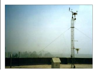
**Measurement Equipment**: Monitors for  $SO_2$  and  $NO_2$ , beta gauge for  $PM_{10}$ , high volume sampler for TSP, dustfall collector and automatic weather station on 10-m mast.
