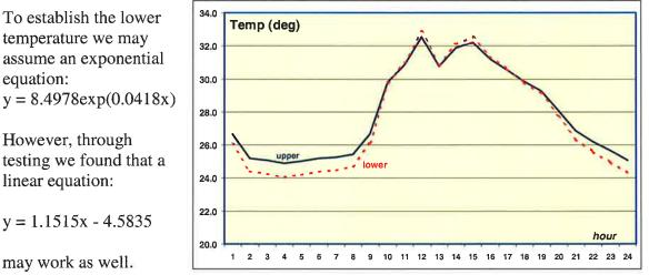
The figure shows a typical diurnal variation of the upper temperature (measured) and the lower temperature estimated.
