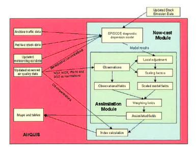
*Figure 8: Data and logical flow diagram showing the AirQUIS data flow structure used for the automatic Now-cast model.*
