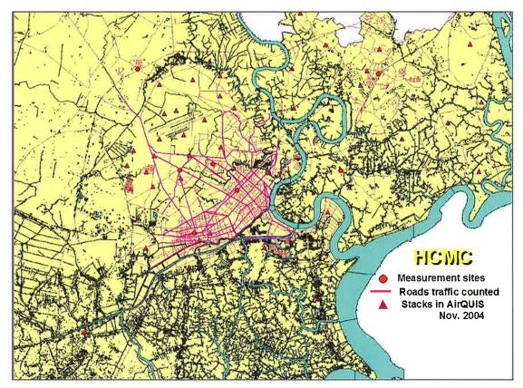
*Figure 3:* The GIS platform in AirQUIS with measurement site positions, roads counted, stacks, rivers and administrative regions. (The stack positions will be verified again).
