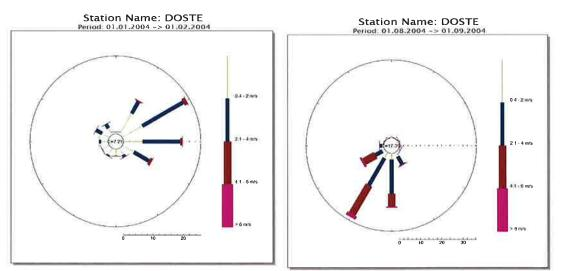
Both the months of January and August 2004 shows NO wind from northerly direction. This error has been present in the data since the measurements started after installations by the Danida project.
