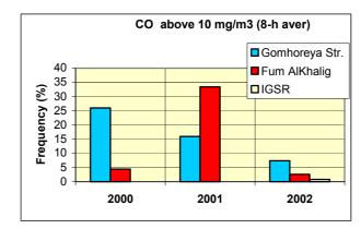
*Figure 6:* The occurrence of 8-hour average CO concentrations above the AQ limit value of 10 mg/m3 measured at one street canyon and two roadside stations.
