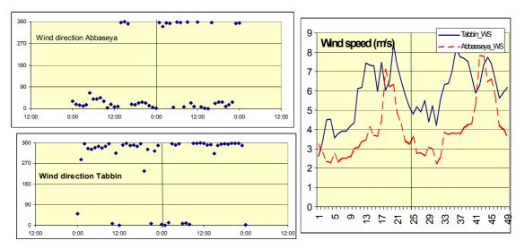
*Figure 3: Wind directions and wind speeds observed at Abbasseya and Tabbin during 9 and 10 October 2003.*
