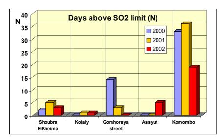
*Figure 5: The number of days when the AQL values for SO*<sub>2</sub> (24-h average) have been exceeded in 2000, 2001 and 2002 at 5 selected sites in Egypt.
