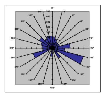
Breuer diagram for PM<sub>10</sub> concentrations at Abbasseya station during 2003
