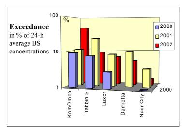
Figure 3: The frequency (in %) of exceeding the Air Quality Limit value of 150  $\mu g/m^3$  as daily average concentration at 5 selected sites in Egypt during 2000, 2001 and 2002.
