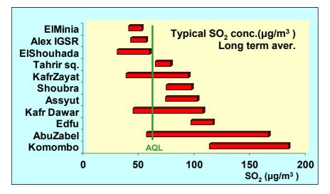
*Figure 6: Typical ranges of long-term average (annual) concentrations of SO*<sub>2</sub> *measured by passive samplers at 11 selected sites in Egypt.*
