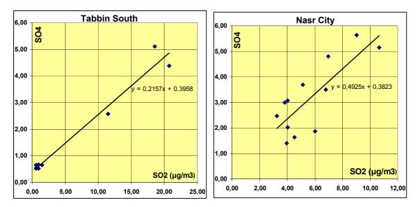
*Figure 1:* Concentrations of SO<sub>4</sub> -S and SO<sub>2</sub> measured on impregnated filters by sequential samplers at Tabbin South and Nasr City, 24 May to 5 June 2003.
