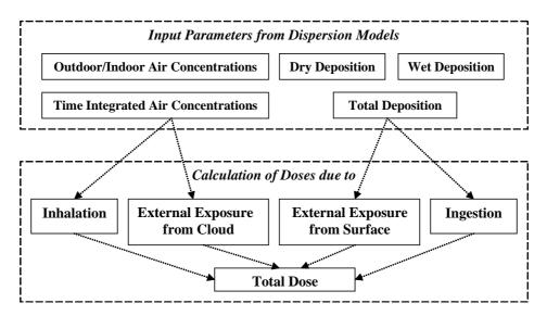
*Figure 7.2: General scheme of individual dose calculations for different groups of the population from radioactive airborne contamination in the ARGOS system.*
