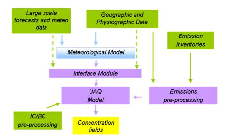
Figure 5.1: Torino's UAQIFS architecture. The prototype system (developed in the FUMAPEX Project) is comprehensive of the meteorological model; in the operational system meteorological forecasts and geographycal/-physiographic data are directly used by the interface module (following green dashed lines).
