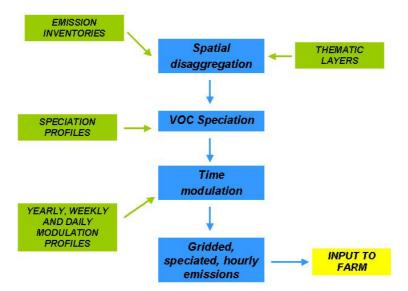
Figure 5.7: Emission Manager flow chart: the pre-processor performs firstly a spatial disaggregation, then applies the VOC speciation and finally the time modulation in order to obtain gridded, speciated and hourly emissions.
