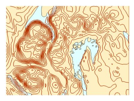
*Figure 2.1:* Topography for the MM5 domain covering the Oslo region (contour interval 50meter).
