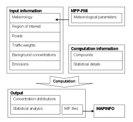
Figure 3.2: The general flow of CAR-FMI. MPP-FMI is meteorological preprocessing, which is replaced by the direct HIRLAM-interface in operative forecasting use; MIF is file format that enables the results of CAR-FMI model to be presented with MapInfo software (GIS, Geographical Information System).
