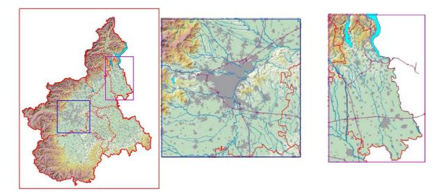
Figure 5.5: Operational system computational domains: the regional domain, with 4 km horizontal resolution and the two nested subdomains (left), respectively the Torino urban area domain (centre) and the Novara urban area domain (right).
