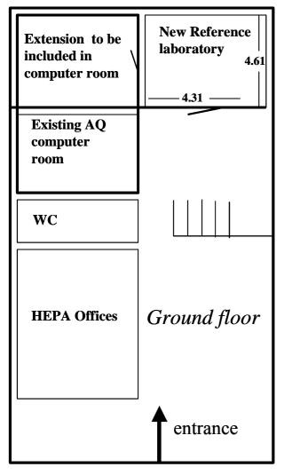
The space for the new Reference Laboratory was inspected. The location is in the first floor of the HEPA building. The size of the room is 4.60m x 4.31 m and the height is 2.15 at the lowest point and about 3.5 m at the highest point. The computer extension room is 3.8 x 4.6 m.
