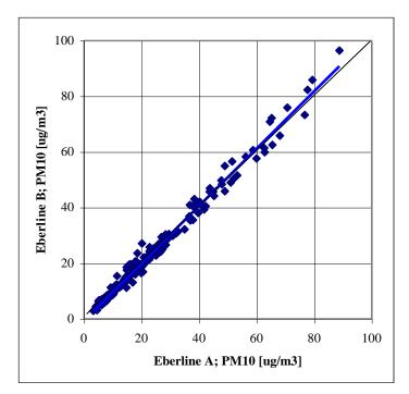
Figure 12. Eberline monitor B compared with monitor A using 23-hour averages.
