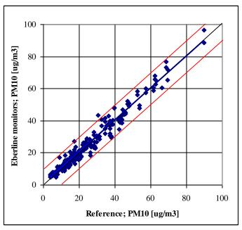
Figure 13. The two Eberline monitors data compared to the  $PM_{10}$  reference data set using 23 hour Eberline monitor averages.
