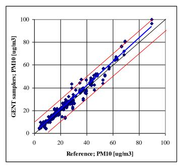
Figure 9. The two Gent samplers data compared to the  $PM_{10}$  reference data set.
