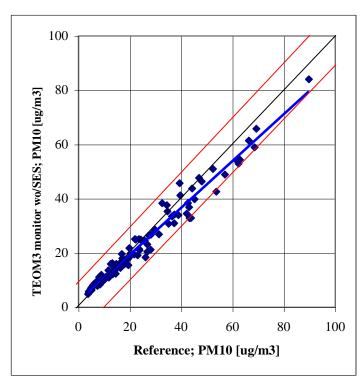
Figure 18. Comparison between the standard type TEOM monitor data and the reference data set.
