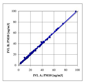
Figure 10. IVL sampler B compared with sampler A.
