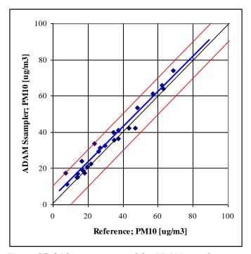
Figure 25. 24 hour averages of the ADAM sampler compared to the  $PM_{10}$  reference data set.  $PM_{10}$  concentrations in  $\mu g/m^3$ .
