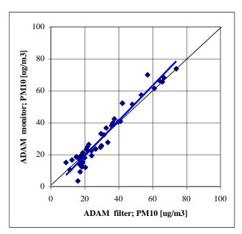
Figure 23. 24 hour averages of the ADAM monitor results compared to the 24 hour ADAM filter results.
