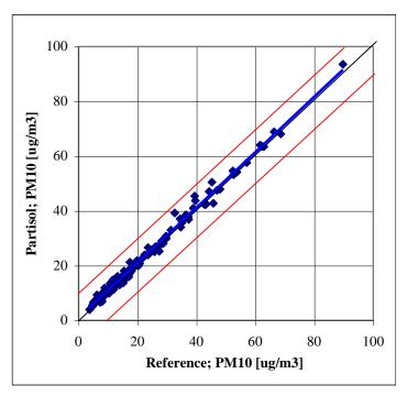
Figure 5. Partisol measurements compared with the reference data set.
