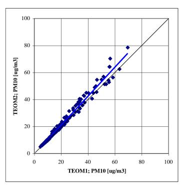
Figure 15. TEOM monitor 2 compared with monitor 1 using 23-hour averages. Both monitors were equipped with nafion driers.
