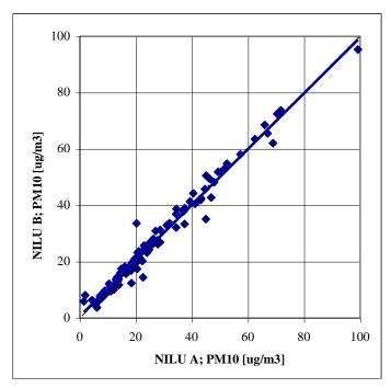
Figure 6. NILU sampler B compared with sampler A.
