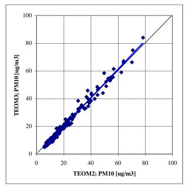
Figure 16. TEOM monitor 3 compared with monitor 2 using 23-hour averages. TEOM 3 was a traditional TEOM running at 50 °C while TEOM 2 was equipped with nafion drier at 30 °C.
