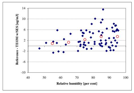
Figure 19.  $PM_{10}$  difference between the reference data set and two nafion drier type TEOM monitors as a function of relative humidity.
