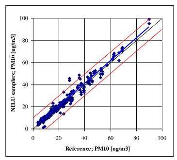
Figure 7. The two NILU samplers data compared to the  $PM_{10}$  reference data set.
