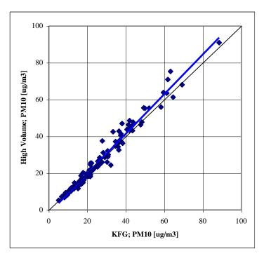
Figure 4. High Volume PM<sub>10</sub> measurements compared with KFG results.
