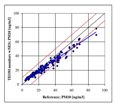
Figure 17. The two nafion drier type TEOM monitors data compared to the  $PM_{10}$  reference data set using 23 hour TEOM monitor averages.
