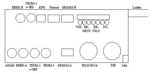
Figure 1. Instrument layout on platform.
