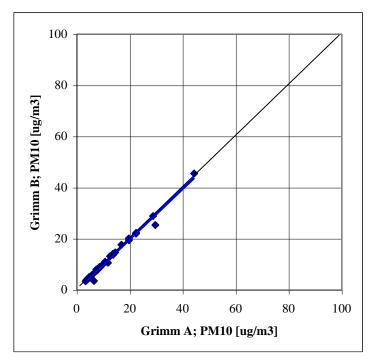
Figure 21. GRIMM monitor A compared with monitor B using 23 hour averages. Data from Elverum wood burning site only.
