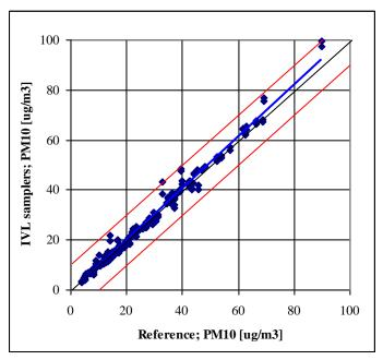
Figure 11 The two IVL samplers data compared to the  $PM_{10}$  reference data set.
