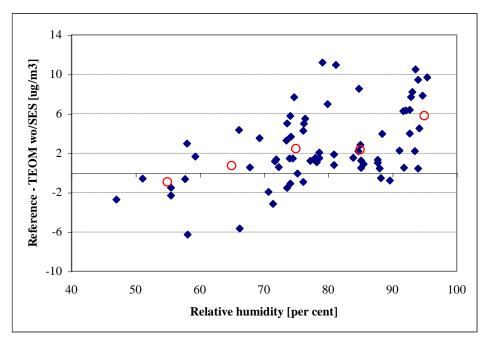
Figure 20.  $PM_{10}$  difference between reference data set and standard type TEOM3 as a function of relative humidity. Circles give the averages of results within 10 % RH class.
