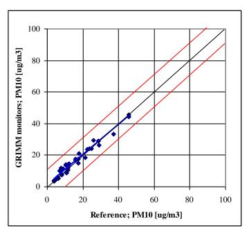
Figure 22. The two GRIMM monitors data compared to the  $PM_{10}$  reference data set using 23 hour GRIMM monitor averages. Data from Elverum wood burning site only.
