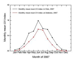
Figure 17: Monthly mean UV doses in 2007 measured with the GUV instruments located in Oslo and Andøya.
