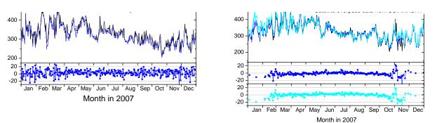
Figure 12: Comparison of ground based total ozone observations with satellite ozone observations. The left panel shows observations from Oslo compared to ozone data from the instrument OMI. The right panel show observations from Andøya compared to ozone data from OMI and SCHIAMACHY. The lower panel shows the percent difference.
