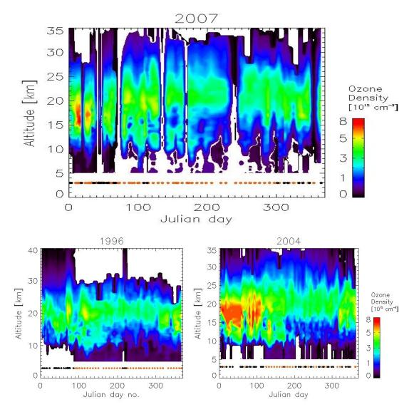
Figure 3: Ozone profiles measured by the ALOMAR ozone lidar and ozone sondes launched in Sodankylä, Finland, in 2007 (upper panel), 1996 (lower left panel), and in 2004 (lower right panel). The black dots at the bottom of the plot mark the times when lidar measurements were performed, while the red dots mark days where data from ozone sondes launched from Sodankylä were used. Between the individual measurements the data were linearly interpolated and smoothed with a one-week median filter.
