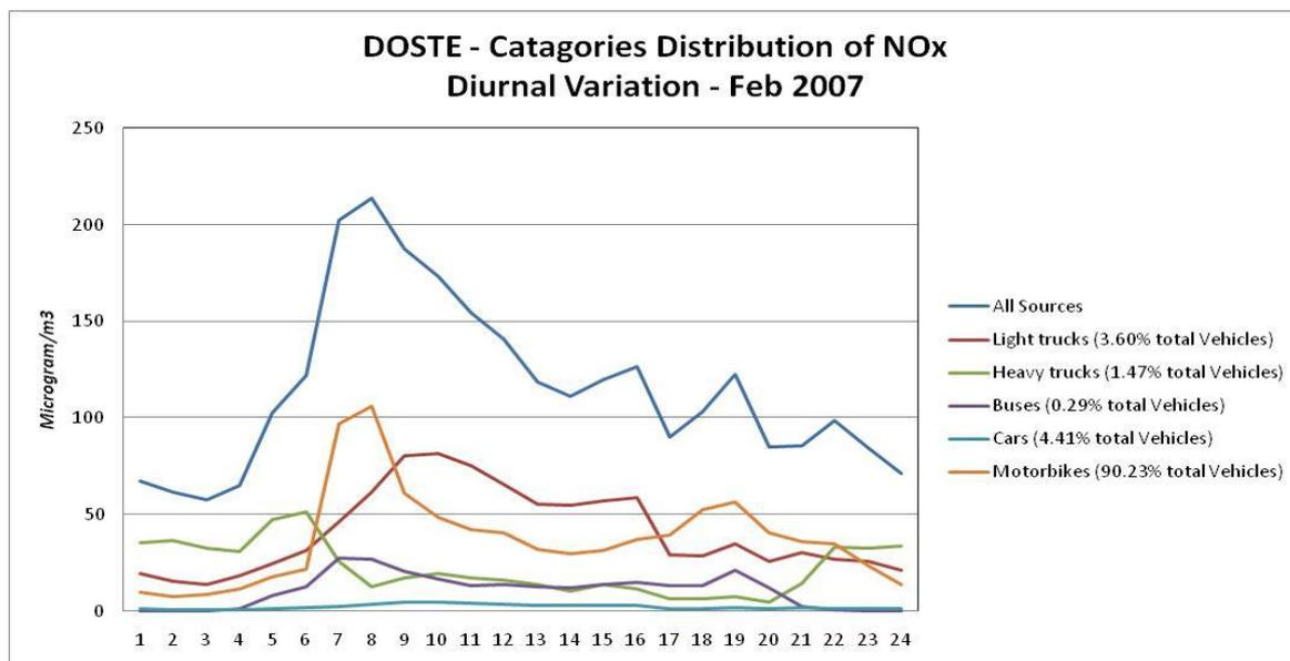
Figure 14: The average diurnal variation of NOx concentrations at Doste presented for 5 vehicle classes and for the total traffic flow (February 2007).
