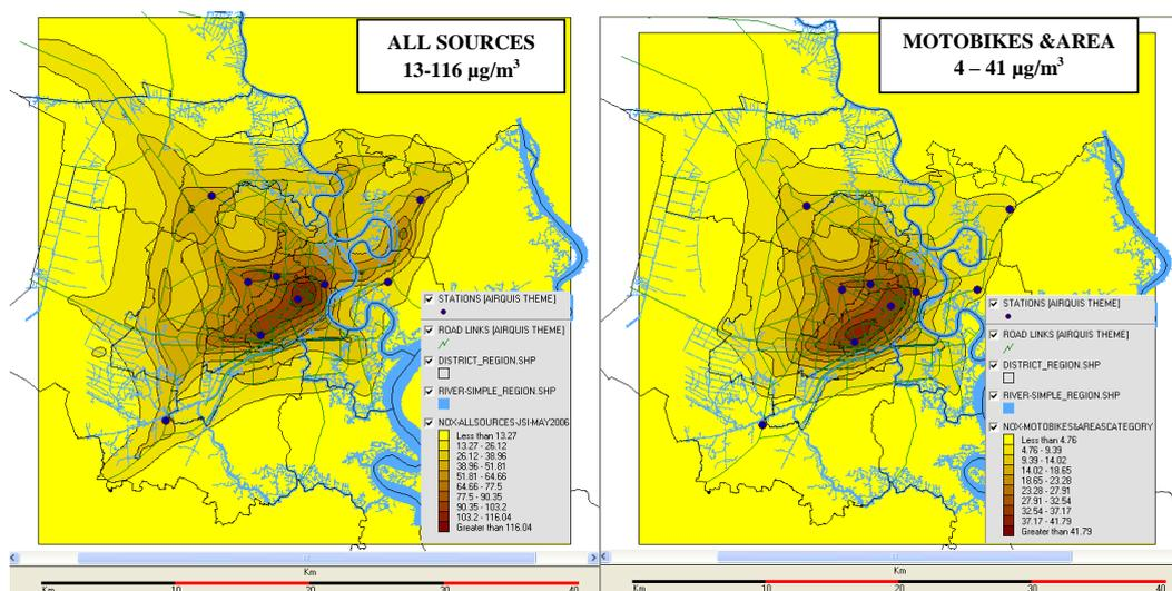
Figure 15: Annual average NOx concentrations estimated for all sources and for emissions from motor bikes in HCMC.
