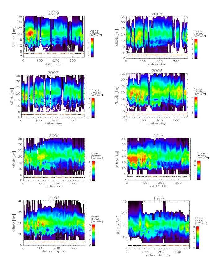
**Figure 4:** Ozone profiles measured by the ALOMAR ozone lidar and ozone sondes launched in Sodankylä, Finland, in 1996 and 2003-2009 (analog to Figure 3).
