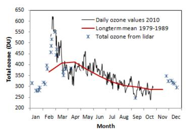
Figure 2a): Daily total ozone values measured at ALOMAR, Andøya, in 2010 by the Brewer, GUV and LIDAR instruments. The use of the different instruments is shown in the lower part of Figure 2a). The red line shows the long-term monthly mean values from 1979-1989.
