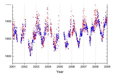
Figure 31: Observations of methane for the period 2001-2008 at the Zeppelin observatory. Blue dots: air mass origin is from a clean sector, red dots: the air mass origin is from a polluted sector.
