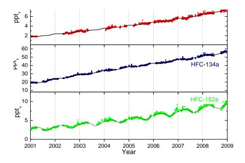
*Figure 18: Daily average concentrations of the monitored CFCs: HFC-125 (red), HFC-134a (dark blue), HFC-152a (green) for the period 2001-2008 at the Zeppelin observatory. The solid lines are modelled background mixing ratio.*
