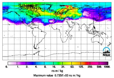
Figure 32: Upper panel: Methane observations for 2008 with an indication of source regions for the elevated episodes. Lower panel: FLEXPART simulations for 16<sup>th</sup> January.
