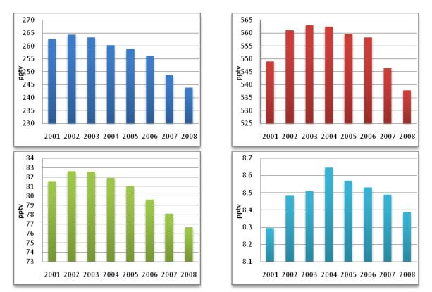
*Figure 15: Development of the annual means all the observed CFCs at the Zeppelin Observatory for the period 2001-2008. Upper left panel: CFC-11, upper right panel: CFC-12, lower left panel: CFC-13, lower right panel: CFC-115.*
