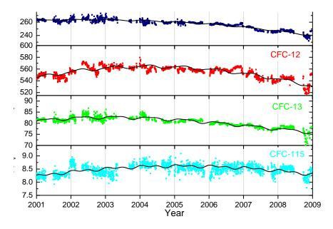
*Figure 14: Daily averaged mixing ratios of the monitored CFCs: CFC-11 (dark blue), CFC-12 (red), CFC-13 (green) and CFC-115 (light blue) for the period 2001-2008 at the Zeppelin observatory. The solid lines are modelled background mixing ratio.*
