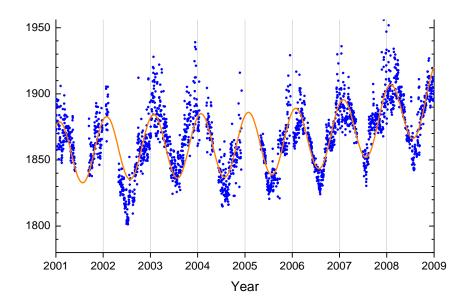
*Figure 3: Observations of daily averaged methane concentrations for the period 2001-2008 at the Zeppelin observatory. Blue dots: observations, orange solid line: modelled background methane mixing ratio.*
