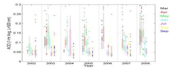
Figure 28: Monthly average aerosol optical depth (AOD at 500 nm) measured in Ny-Ålesund during the sunlight time periods in 2002 - 2008. On each box, the central mark is the median, the edges of the box are the 25th and 75th percentiles, the whiskers extend to the most extreme data points not considered outliers, and outliers (in terms of monthly averages, although not considered outlier in terms of pollutions events with high aerosol loads) are plotted individually.
