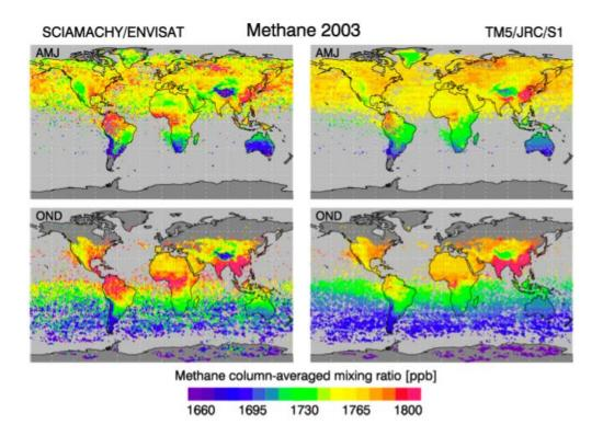
*Figure 33: 3-month (seasonal) dry air column averaged XCH4 mixing ratios (ppb) determined from SCIAMACHY. Left-hand panels: SCIAMACHY measurements. Right-hand panels: TM5 model.*
