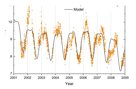
Figure 9: Observations of methyl bromide,  $CH_3Br$ , for the period 2001-2008 at the Zeppelin observatory. Dots: daily averages mixing ratios from the observations, solid line: modelled background mixing ratio.
