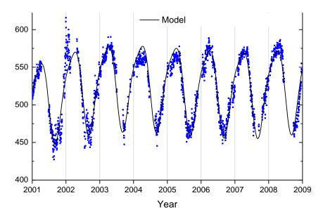
Figure 7: Observations of methyl chloride,  $CH_3Cl$ , for the period 2001-2008 at the Zeppelin observatory. Dots: daily averaged concentrations from the observations, solid line: modelled background mixing ratio.
