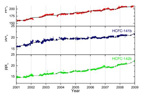
Figure 16: Daily average mixing ratios of the monitored HCFCs: HCFC-22 (red), HCFC-141b (dark blue) HCFC-142b (green) for the period 2001-2008 at the Zeppelin observatory. The solid lines are modelled background mixing ratio.
