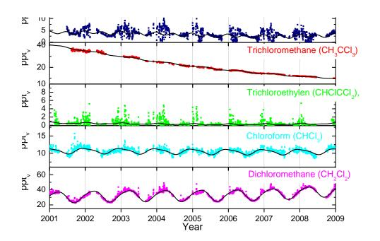
Figure 22: Daily average concentrations chlorinated hydrocarbons: From the upper panel: Perchloroethylene (dark blue) Trichloromethane (red), Trichloroethylen (green), Chloroform (light blue) and Dichloromethane (pink) for the period 2001-2008 at the Zeppelin observatory. The solid lines are the modelled background mixing ratio.
