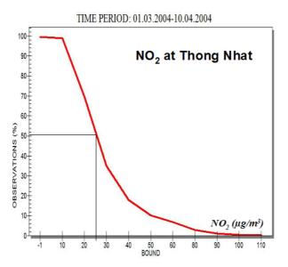
*Figure 22:* The cumulative frequency distribution of NO2 for one year of measurements at Thong Nhat.
