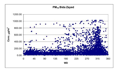
*Figure 26:* Scatter plot of PM10 concentrations measured at Bida Zayed as a function of wind direction.
