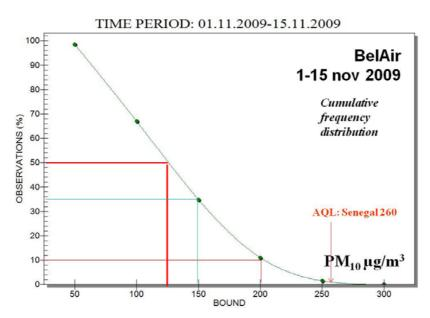
*Figure 12: Cumulative frequency distribution for PM10 measured at BelAir during 1 to 15 November 2009.*
