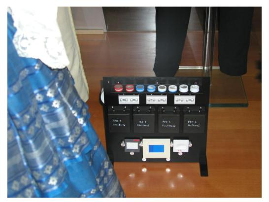
Figure 2.60: The MASTER Field test set up on location in a museum, with exposure of the EWO dosimeters, gas sampling with passive samplers, exposure of organic materials and climate measurements. The calibration of the measured effects of the environmental parameters on the EWO-G dosimeter exposed on location, compared to that on organic museum objects was performed using literature values for observed effects of the parameters on organic museum objects.
