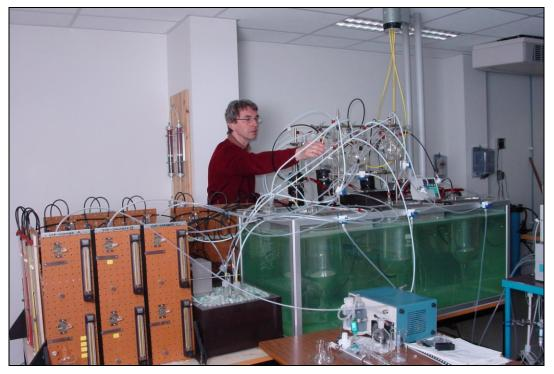
Figure 2.17: The climate chamber at NILU used for testing the EWO- G dosimeters.
