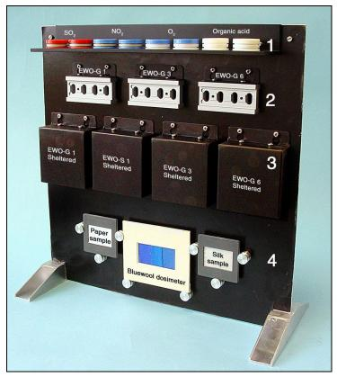
Figure 2.27: The MASTER field test exposure rack.
