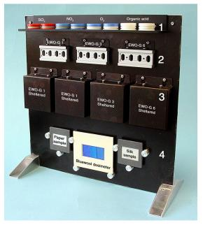
*Figure 2.2: Picture: Dosimeter, - blue wool? The exposure rack for dosimeter, object and pollutant monitoring in the MASTER project.*
