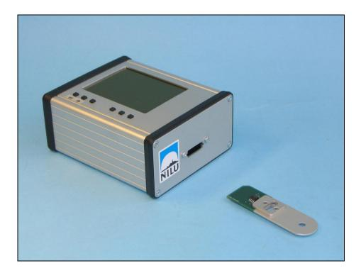
*Figure 2.13: The first prototype of a portable measurement instrument for the EWO-G dosimeter.*
