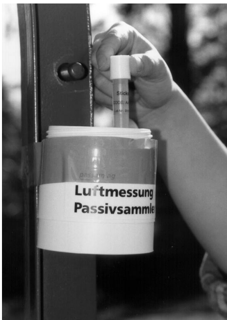
Figure 1: Left: Passive sampler (Palmer's tube) and housing from Passam ( www.passam.ch ). Right: Passive sampler (badge) with housing from Ogawa ( www.ogawausa.com ).
