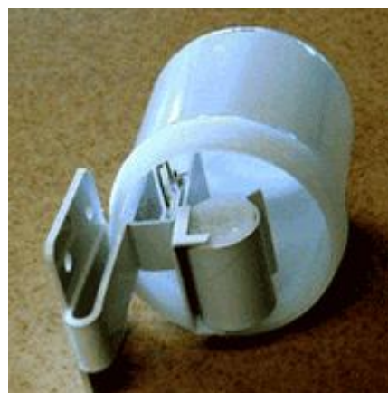
Figure 1: Left: Passive sampler (Palmer's tube) and housing from Passam ( www.passam.ch ). Right: Passive sampler (badge) with housing from Ogawa ( www.ogawausa.com ).
