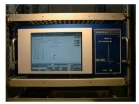
Figure 4: For monitoring of Benzene-Toluene-Xylene (BTX) components a Syntech Spectras GC-855 (Synspec, Groningen, The Netherlands) monitoring device was used. Figure reproduced with courtesy of Synspec, Groningen, NL As representative volatile organic pollutants, Benzene-Toluene-Xylene (BTX) were also analysed in/ above soil samples, collected in parallel with the soil material dedicated for PAH analysis (see above). All soil samples were, thus, collected in duplicate.
