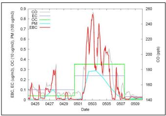
Figure 10: Observations of CO, aerosol elemental carbon (EC), aerosol organic carbon (OC), total particulate matter (PM) and absorbing black carbon in aerosols (EBC) at Zeppelin observatory. (From Stohl et al. 2007)
