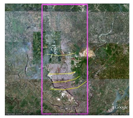
Figure 5: Targeted transect lines (yellow lines) to locate passive sampling sites along. Pink rectangle signifies the modelling grid area for the BAPMAN project. (Background Imagery Source: Google Earth).
