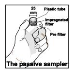
*Figure 6: Ilustration of passive sampler.*
