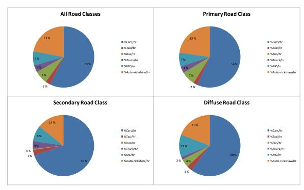
Figure 44: Vehicle class distributions for each road class.
