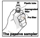
These samplers have been used by NILU in a number of studies (Hak, 2010; Hak and Sivertsen, 2010). For sampling of gases they include an impregnated filter inside a small plastic tube. To avoid turbulent diffusion inside the sampler, the inlet is covered by a thin porous membrane filter. Gases are transported and collected by molecular diffusion.
