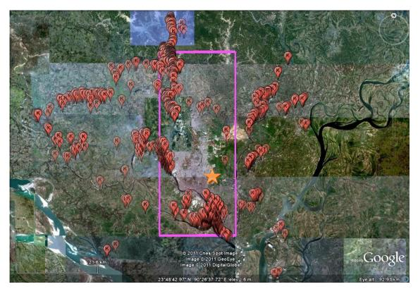
Figure 1: Map of 983 Brick Kilns in greater Dhaka area. Pink rectangle signifies the modelling grid area for the BAPMAN project; Dhaka city center is marked by the orange star. (Background Imagery Source: Google Earth).
