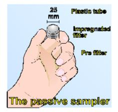
A sensitive diffusion sampler for sulphur dioxide ( $SO_2$ ) and nitrogen dioxide ( $NO_2$ ) in ambient air has been used in several investigations to undertake a screening of the spatial concentration distribution.
