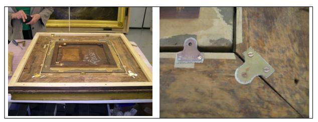
*Figure 26:* Back of Rossetti painting with hardboard backing removed. Top right hand corner shows crystals mounted in steel frame and top left corner shows lead coupon and A-D strip (Left). Reverse of Rossetti painting showing deposits on brass plates (Right).
