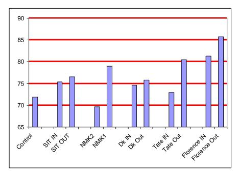
Figure 52: Graph shows the plot of  $Tg(^{\circ}C)$  vs. sites. IN = Inside microclimate frames. OUT = outside microclimate frames.
