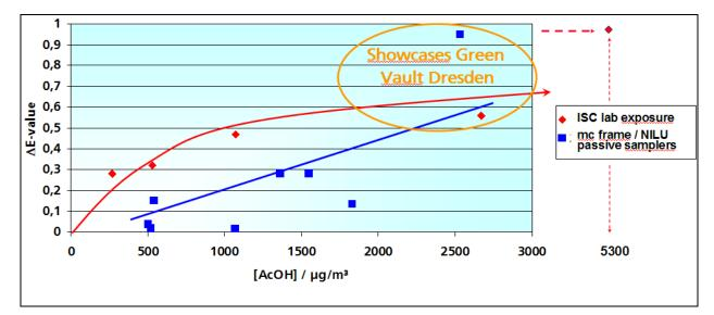
Figure 10: Environmental Glass Slide Dosimeters: correlation of ∆E-values (3 months exposure) after acetic acid exposure vs. acetic acid concentration (all available data).
