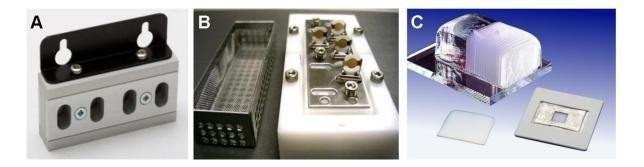
Figure 4: The main dosimeters used in the PROPAINT project: A. The NILU EWO (Early Warning dosimeter for Organic materials). B. The Birkbeck PQC (Piezoelectric Quartz Crystal) dosimeter and C. The Fraunhofer ISC GSD (Glass Slide Dosimeter).
