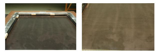
Fig. 4. Whitish deposits on inside of glass of the microclimate box, photographed (on a black cloth), 11 July 2007.
