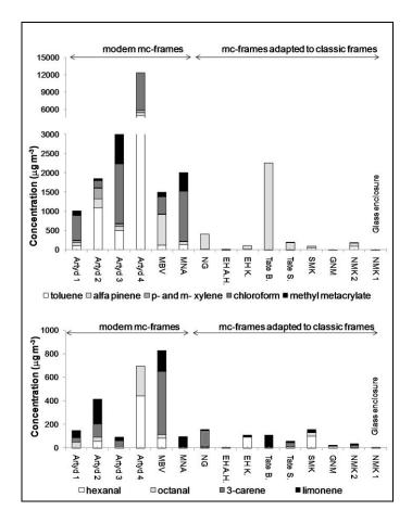
Figure 20: Concentration of specific VOC inside "modern" microclimate frames and microclimate frames adapted to "historic" frames including the glass enclosure. For location abbreviations see Table 3 and table in Figure text 12.
