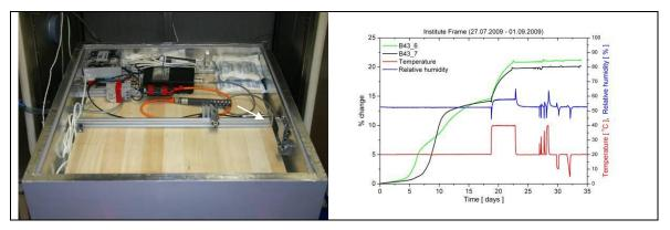
Figure 24: The position of the L-PQC dosimeter (crystals in flat silver holder) is shown using the arrow (left). The green and black traces show the change (%) in the crystals on exposure. The change occurs over the first 10/15 days. After 20 days the conditions in the microclimate chamber were changed (RH,T) (Right).
