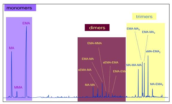
Figure 40: Pyrogram of Paraloid B72 at 600°C.
