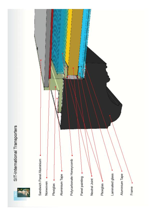
Figure 64: Microclimate frame constructed by SIT.
