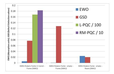
Figure 15: Results from exposures of the EWO, GSD. L-PQCs and RM-PQCs inside and outside the SMK2 microclimate frame (Table 23). The units for the L-PQC and RM-PQC are % change and 1000\*f/F (= relation between the frequency shift and the original coated crystal frequency), respectively.
