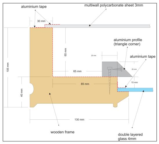
Figure 60: Microclimate frame for "epitaph of Jan Shupecki" (section).
