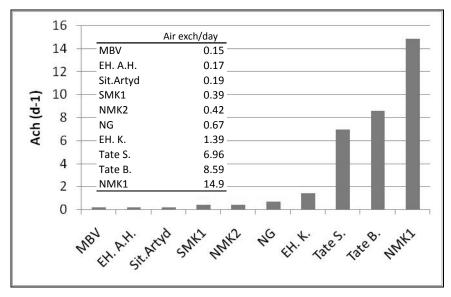
*Figure 23: Air exchange rate of PROPAINT-microclimate frames. For location abbreviations see Table 3 and table in Figure text 12.*
