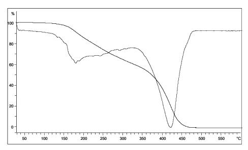
*Figure 41: Thermogravimetric graph for MS2A (continuous line) and relative derivative (dashed line).*
