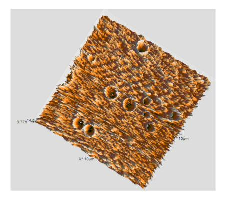
Figure 53: AFM image (10  $\mu$ m x 10  $\mu$ m) of B72 exposed to NO<sub>2</sub> (4ppm for 27 days) at 80 % RH.
