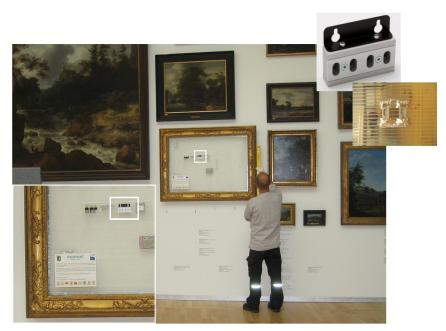
*Figure 5:* The EWO dosimeter developed at NILU, exposed at Statens Museum for Kunst, Copenhagen, DK. Upper Right; the holder for up to four dosimeters, below the miniaturised holder for one dosimeter.
