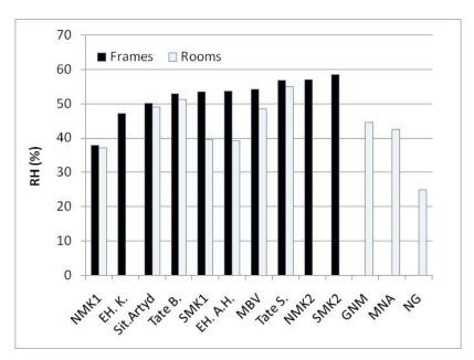
Figure 22: Mean relative humidity measured inside and outside the microclimate frames for paintings. For location abbreviations see Table 3 and table in Figure text 12.
