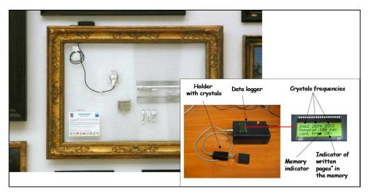
*Figure 7: The PQC dosimeters for continuous operation, developed by Birkbeck, exposed at Statens Museum for Kunst, Copenhagen, DK.*
