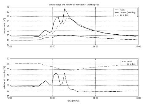
Fig. 9. Temperature and relative humidity measurements from a test painting in microclimate box exposed to direct sunlight, 22 January 2005. (The anomalous low relative humidity of the air in the box (35%) in the lower spectrum was due to insufficient conditioning of the test painting prior to placement in the microclimate box (from Baan and Van Duijnhoven 2005, p. 51)).
