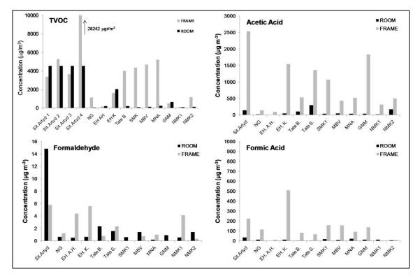
Figure 19: Total concentration of volatile organic compounds (TVOC), acetic acid, formic acid and formaldehyde measured inside and outside microclimate frames. For location abbreviations see Table 3 and table in Figure text 12.
