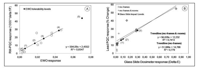
Figure 17: Correlation between dosimeter responses in microclimate frames and rooms. A: EWO and RM-PQC with locations tolerability levels (Figure 14C and A). B: GSD and L-PQC with impact levels (Figure 14D and Figure 15B).
