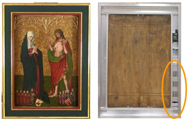
*Figure 35: National Museum in Krakow (PL) "New microclimate frame". The varnish samples are exposed in the darkness.*
