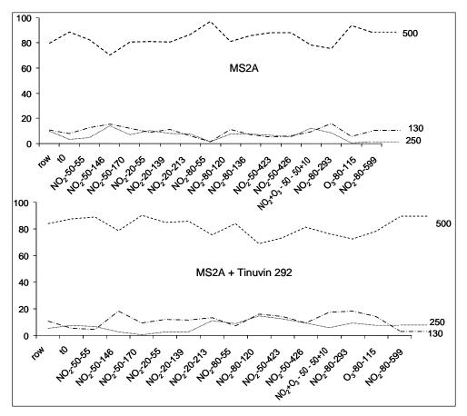
*Figure 43: Comparison of the relative amounts of monomers, dimers and macromolecular fraction evaluated as the sum of peak areas in chromatograms corresponding to the thermal desorption at 130 °C, at 250 °C and pyrolysis at 500 °C, respectively.*
