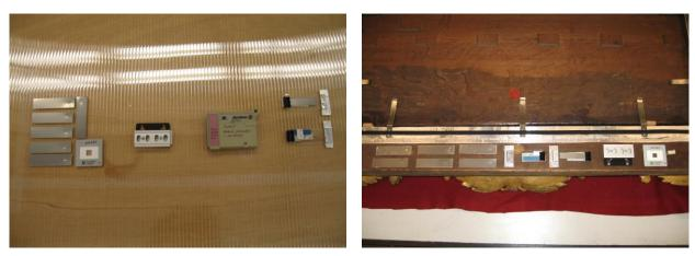
*Figure 32: Statens Museum for Kunst, Copenhagen (DK): Inside (left) and outside (right) the frame. The varnish samples are exposed in the darkness.*
