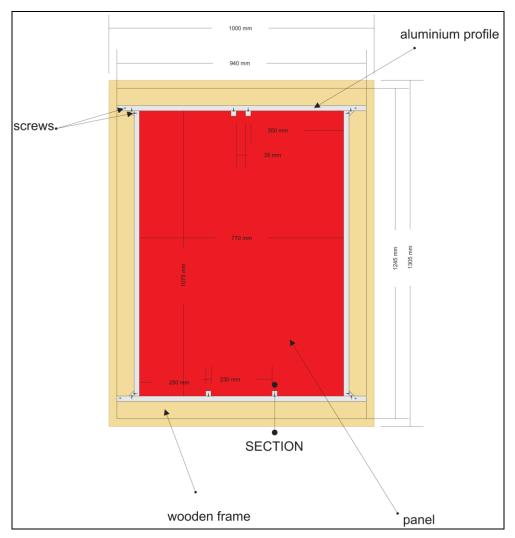
Figure 59: Microclimate frame for "Epitaph of Jan Słupecki" (back).
