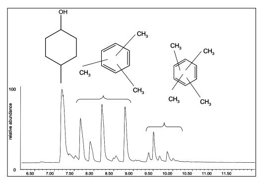
*Figure 44: GC-MS chromatograms of MS2A resin of the varnish sample NO2-80-599 desorbed at 130°C.*
