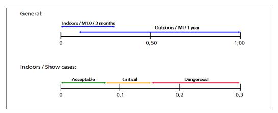
Figure 9: Environmental Glass Slide Dosimeters (type M1.0 and MI): range of exposure results (ΔE-values) and related evaluation criteria after 3 month exposure (see also Figure 14).
