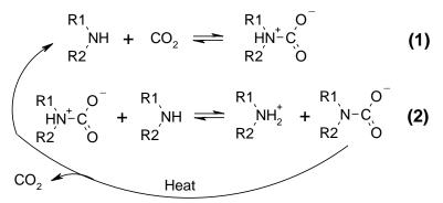
Figure 2. The chemistry behind amine based CO<sub>2</sub> capture.
