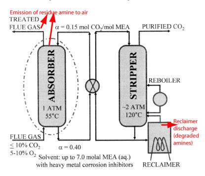
Figure 5. Sources of amine discharge in the CO<sub>2</sub> capture process.
