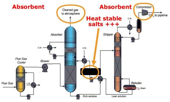
Figure 3. The CO<sub>2</sub> capture process.
