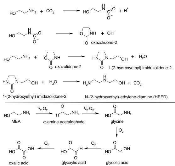
**Figure 6.** Some transformation products of MEA following reactions with  $CO_2$  (top) and  $O_2$  (bottom). The figure is from Bello and Idem, 2005).
